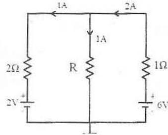
70. The value of the load resistance ( $R_L$ ) to draw the maximum power in the circuit shown in the figure is
